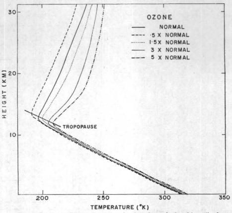
Fig. 7. Radiative equilibrium temperature for given changes in the mixing ratio of ozone
