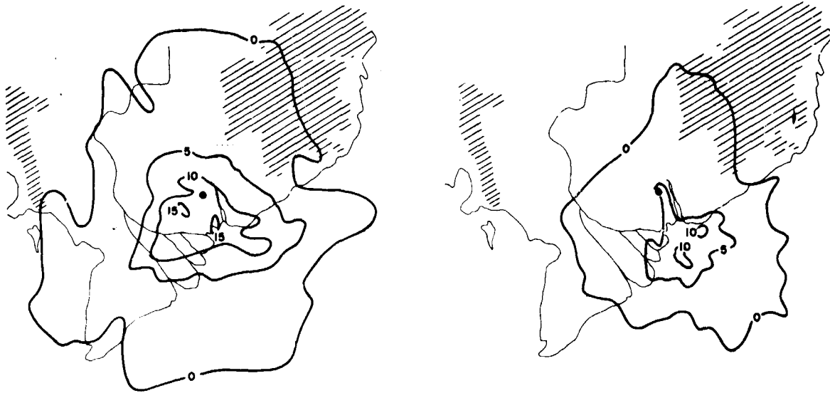
Figure 47. Distribution of All Echoes on Tertile 1 and 3 Days. 06-11 LT Tan Son Nhut. Hilly areas are hatched, radar is located at the dot.
